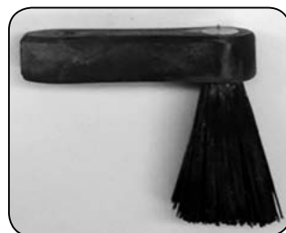
Level 3- Excessive splay, replace to prevent stalling of wiper
